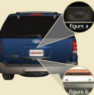
To unlatch the liftgate glass, push the button (figure a) under the center of the license plate lamp shield.
